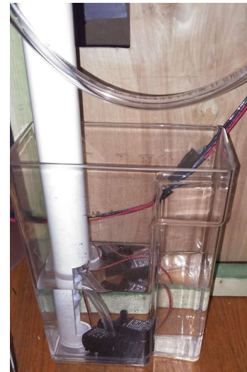
Figure 3: View of front of reservoir showing both pumps with tubing passed through PVC piping into the enclosure.
