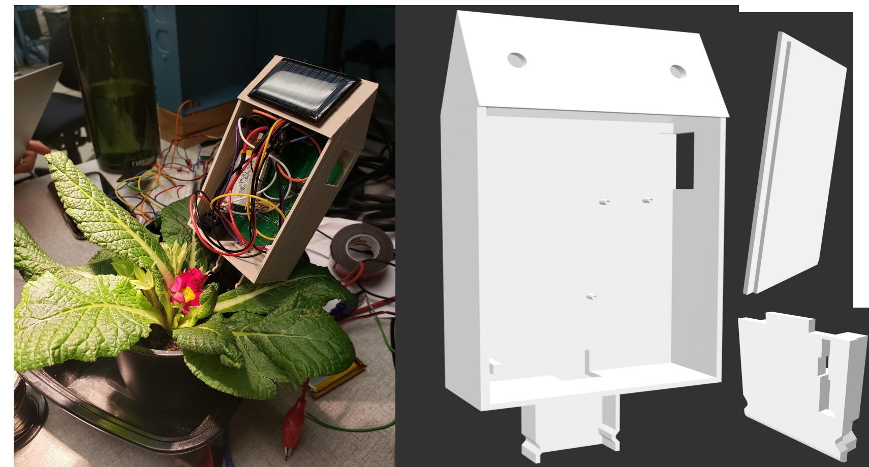
Figure 1: The real-world prototype of Clover, being tested under a halogen lamp in the SDP Lab (left image), and the enclosure 3D CAD designs (right images).
