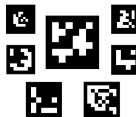
Fig. 4. Examples of ArUco markers. Each marker is unique by its size and pattern. Each pattern has an internal binary matrix that determines its identification. All markers have a black border surrounding the image of the white pixel patterns. Image courtesy of docs.opencv.org/3.1.0.
