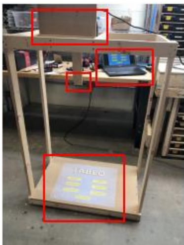
Fig. 3. Tablo, final product. Highlighted components are (from bottom to top): the surface area on which users can play games, the camera for tracking motion of users’ controllers, our laptop for simulation of games, and the projector to display games. This apparatus was placed upon a table, such that the surface area on which users play the game can be played at a typical height of a table. The supportive, wooden beams are necessary to allow for players to experience playing board games wirelessly and digitally, as we could not mount the projector on the ceiling of the common room.
