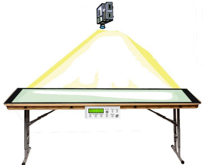
Fig. 1. Depiction of our gaming system. Projector and camera will be hung over user’s table, about 5 feet to 6 feet above their table. The control box, where our PCB board will be used, is mounted on the edge of the table to allow users to perform necessary functions such as: pausing the game, resetting the game, or switching the amount of players in the game, just to name a few.
