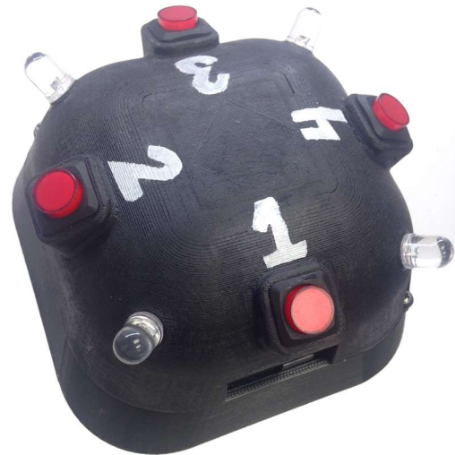
Fig 2. Picture of the final Table Unit Design. There are four LED push buttons on each side and four IR LEDs on each corner. The front panel houses the ON/OFF switch and microUSB port for charging.
