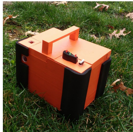
Figure 14: Transmitter Box with Alignment button and LEDs
