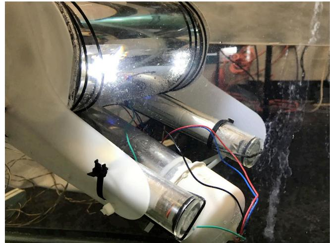
**Fig. 9.** The piston ballast system installed and maintaining depth of the ROV in a water tank without vertical motor input.
