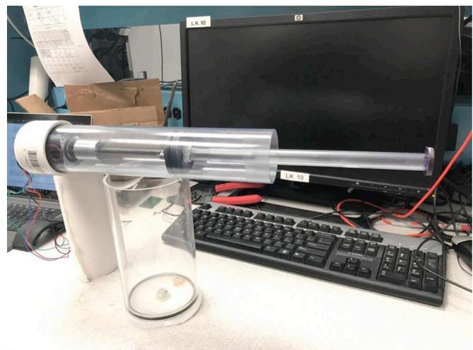
**Fig. 7.** Fully assembly of the piston ballast used to control the depth of the ROV.
