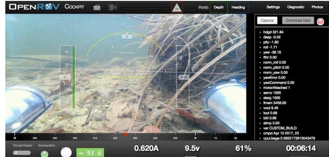
**Fig. 3.** Cockpit is a user interface that the user access through a personal computer to stream live video footage from the onboard camera and control the ROV.
