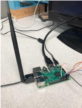
**Fig. 4.** The Raspberry Pi 3 Model B is equipped with a USB wireless antenna to allow it to emit a wireless signal. This allows the user to control the ROV wireless
