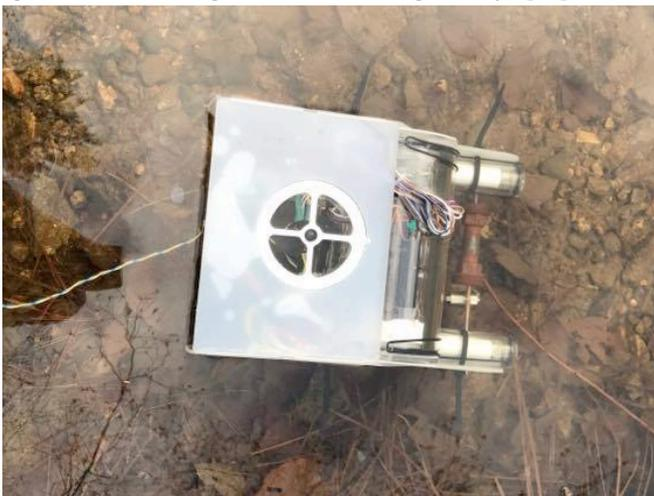
**Fig. 6.** Topside picture of the ROV at Puffer's pond. The underwater drone was taken to a pond environment to test for leakages.
