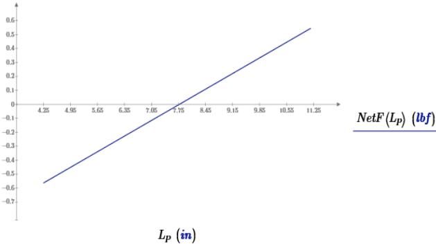
**Fig. 8.** Plot depicting the buoyant force generated by the piston ballast. Negative values to the left indicate the ROV is sinking, while positive value to the right indicate that the ROV is generating lift from fluid displacement.
