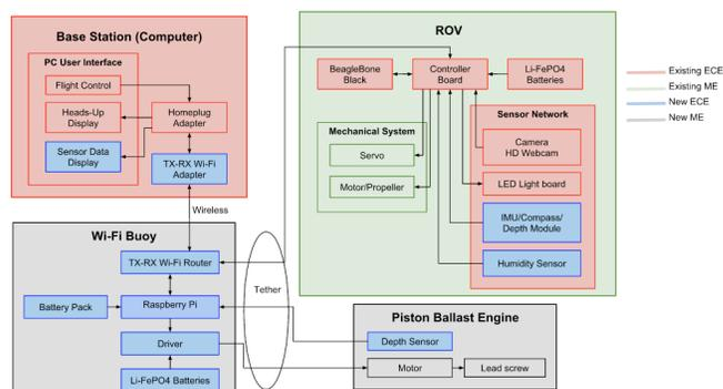
Fig. 2. System block diagram consisting of four major subsystems; base station, Wi-Fi boat, ROV, and piston ballast engine.
