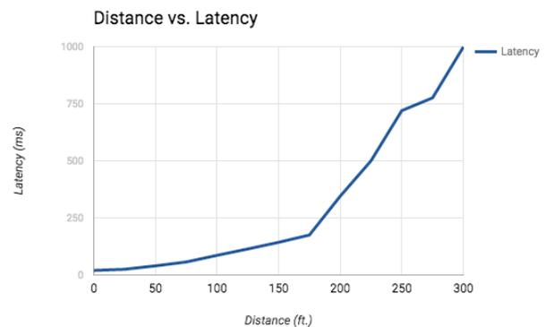
**Fig. 5.** Plot showing the latency of the Wi-Fi setup as the distance of the connection increases.
