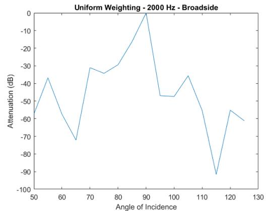
Fig. 16. Experimental Response to 2000 Hz, with Uniform Weighting
