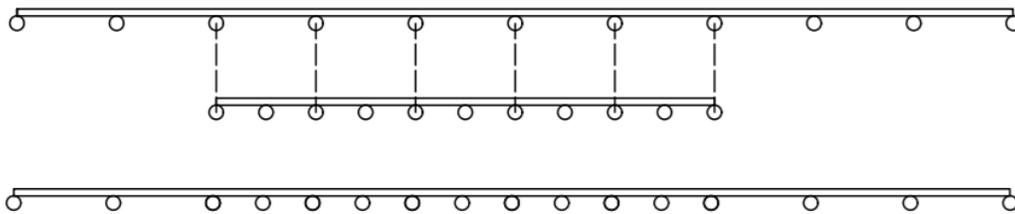
Fig. 10. The Array Geometry for the new Earbeamer array. 16 microphones are shared between a [600,1200] band with  $d= 7\text{cm}$ , and a [1200,2400] band with  $d = 14\text{cm}$
