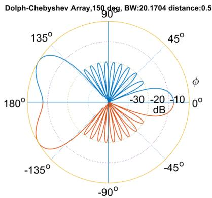
Fig. 12. Earbeyer Array with Dolph Chebyshev weighting, steered towards 150°, with microphone distance  $\lambda/2$
