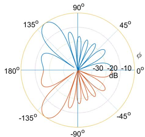
Fig. 7. Array Power gain  $|A(\phi)|^2$  for an array of 8 elements, spaced one-half a wavelength apart, with each microphone equally weighted and steered towards 125°
