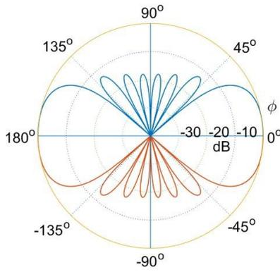
Fig. 4. This is the array response when the elements are steered toward  $180^\circ$  or  $0^\circ$ . You cannot amplify one direction without also amplifying the other direction
