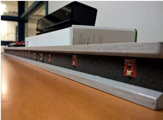
Fig. 20. The final array system and Kinect. Microphones sit on a foam layer, and connect to a PCB inside the housing. When in use, a black cloth sleeve is placed over the array to hide the microphones
