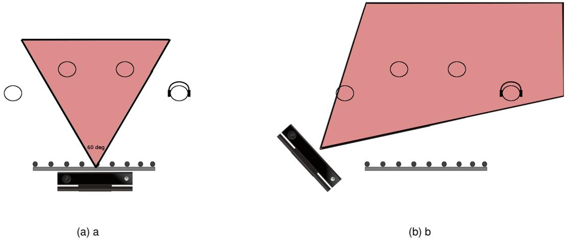
Fig. 22. The Angle of View is too narrow to adequately cover a room, so the Kinect must be offset from the microphone array to identify all possible targets
