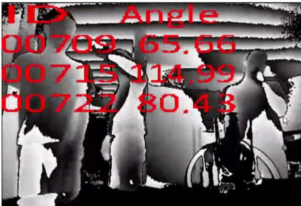
Fig. 13. Plot of depth data returned from Kinect, showing the output of the MDR demo. For each tracked individual, the user ID and angular displacement is printed
