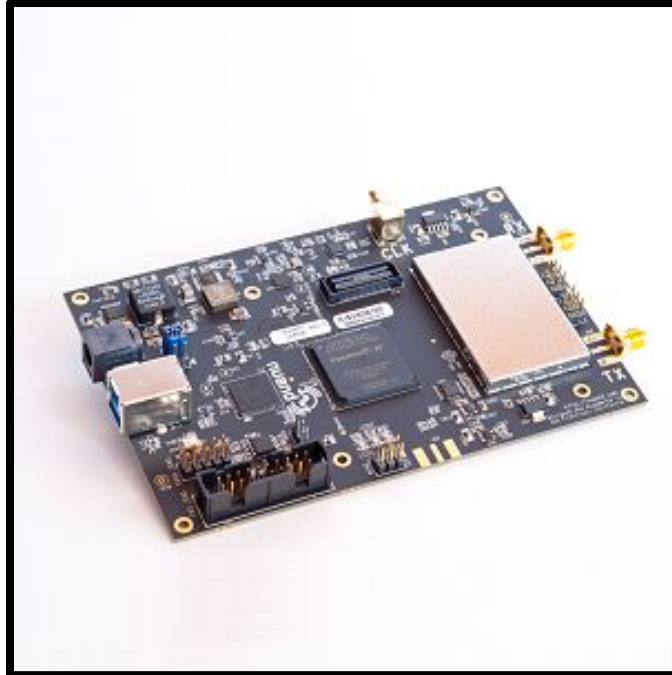
bladeRF X40 Weight: 80g Size: 3.5" x 5.0" Output: +6 dBm
