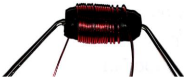
Figure 4. Inductor Wrapped in Magnetic Wire
