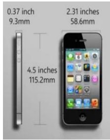
Figure 14. Dimensions for standard iPhone 4
