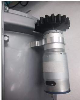
Figure F: Motor and Pinion Gear Mounted to SKLZ Unit
