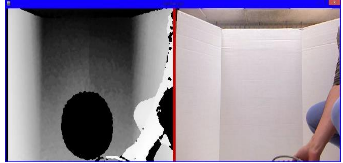
Fig. 3. IR Interference with Kinect 3D Depth map
