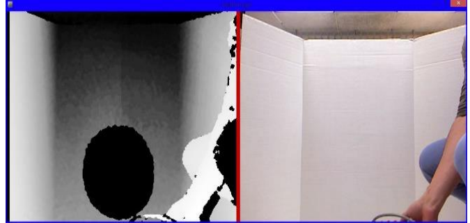
Fig. 3. IR Interference with Kinect 3D Depth map
