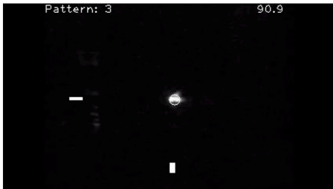
Fig. 3. Visual output of IR tracking. The beacon can be seen in the middle of the screen. The pattern detected is in the upper left corner. The upper right corner displays the frame rate of the camera. The bars at the bottom and left represent the amount the motors need to move the system.
