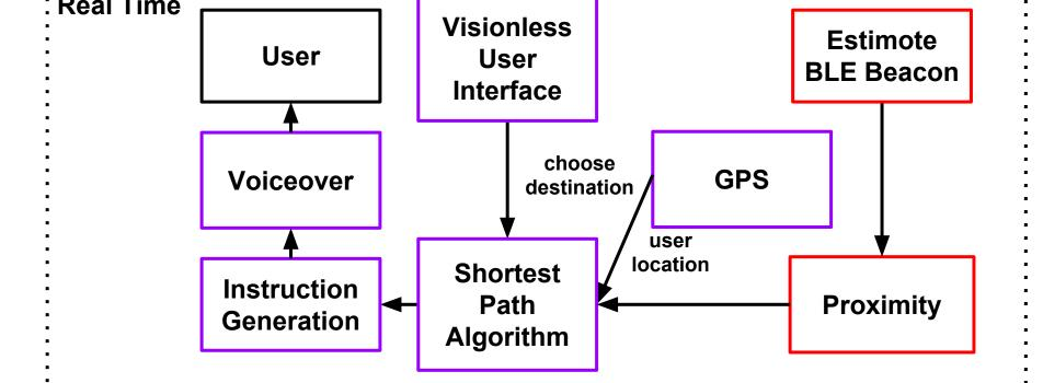
The indoor system determines the user's location and shortest path to their destination using BLE beacons. The outdoor system uses GPS to do the same. Instructions are generated to help the user navigate. BLE beacons are used to transition between the outdoor and indoor environments. BLuEye will notify the user when they have reached their destination.
