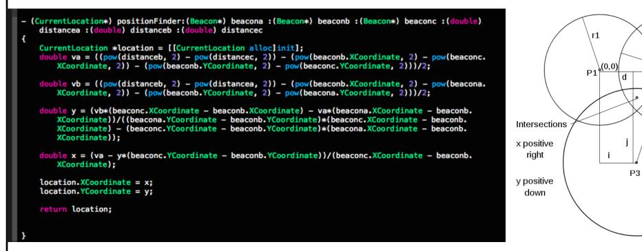
Once the coordinates of the user are found by this algorithm, they are used to determine the closest node on the path. We can determine direction of the user by comparing this node to their destination node. To determine when the user has reached their
