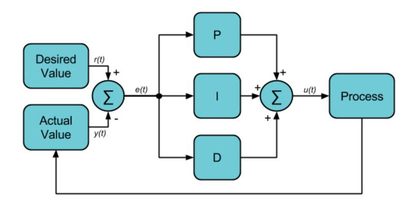
To perform flight stabilization, we utilized a majority of the sensors onboard the APM2.6 Flight Control Board, including its accelerometer, gyroscope, and barometer. Measurements from each of these sensors is fed into a PID (proportional, integral, derivative) feedback controller along with the desired values. The PID controller determines the error between desired and actual values, and returns the change in throttle to the main flight software. FollowMe (GPS Tracking)
