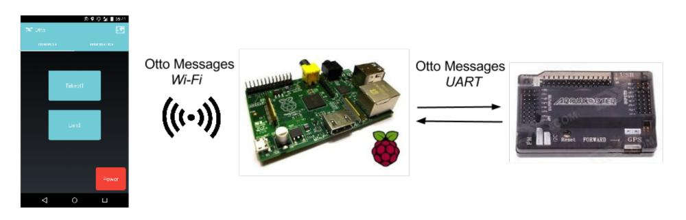
The messaging protocol is built on top of a UDP connection over Wi-Fi @2.4Ghz and a UART communication link which has a baud rate of 115200. Messages are ASCII encoded and they include a start of message character, message identifier, payload and an end of message character. This messaging protocol enables the user to initiate takeoff, land and view live diagnostics.
