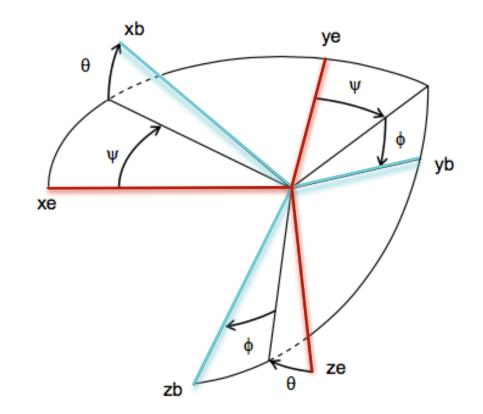
This is Otto's navigation system; the inputs are the drone's and user's GPS coordinates and the output is pitch, roll, and yaw commands to be used to fly the drone to the target. First, the orientation of the drone must be translated from its local body axis system to the global earth axis coordinates (seen above), it is done using the direction cosine matrix (dcm). The commands are calculated through a PID feedback controller. The heading is obtained from the onboard magnetometer (compass).
