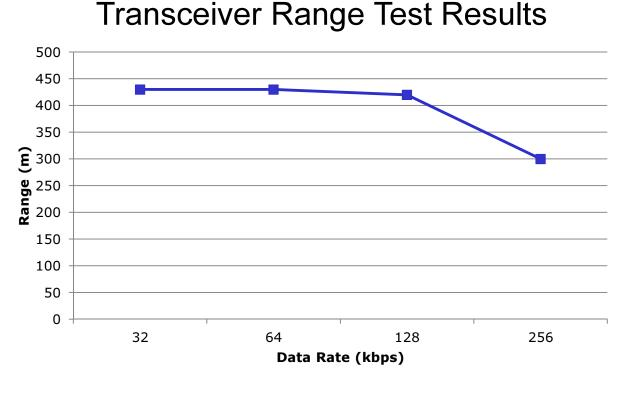
Tested with 4.5v power supply and quarter-wavelength wire antennas
