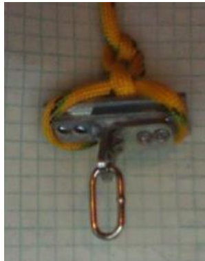
Test load cell taken from luggage scale
