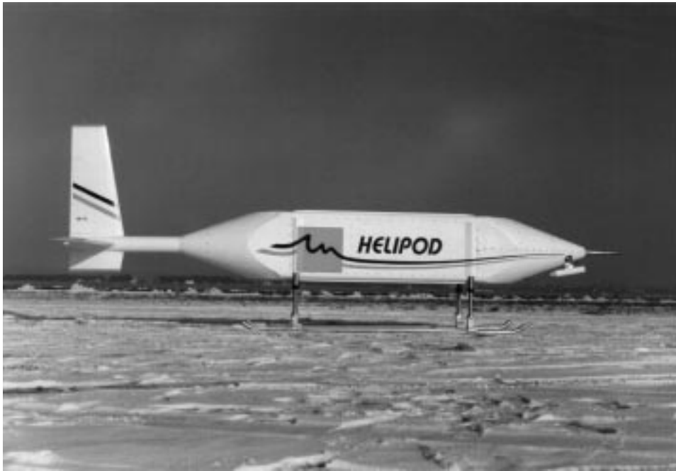
Figure 5. The helicopter-borne turbulence measurement system HELIPOD. The photograph was taken during a field experiment in the Arctic.
