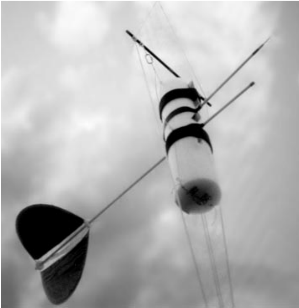
Figure 4. The CIRES sensor payload, which includes a Pitot tube and a thermocouple sensor.
