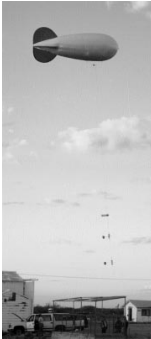
Figure 3. The CIRES/USAF sensor array, suspended below the CIRES blimp. The uppermost package is the basic meteorology payload, in the middle is the USAF sensor package (hot-wire and cold-wire sensors), and at the bottom there is the CIRES sensor package (thermocouple sensor and Pitot tube). The CIRES package hangs 2.95 m below the basic meteorology payload.
