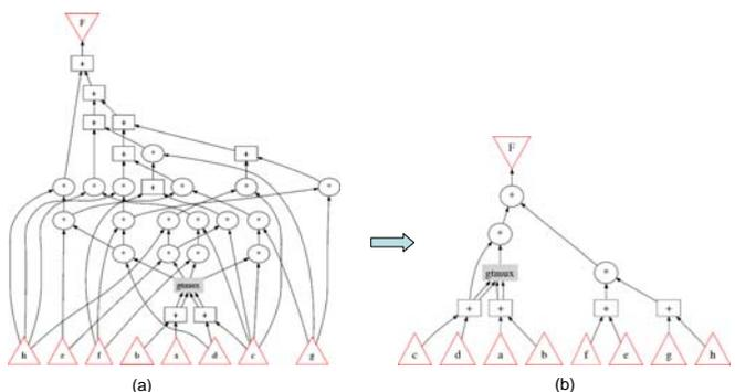
Fig. 5 TD Network optimization: (a) initial TD network, (b) optimized DFG
