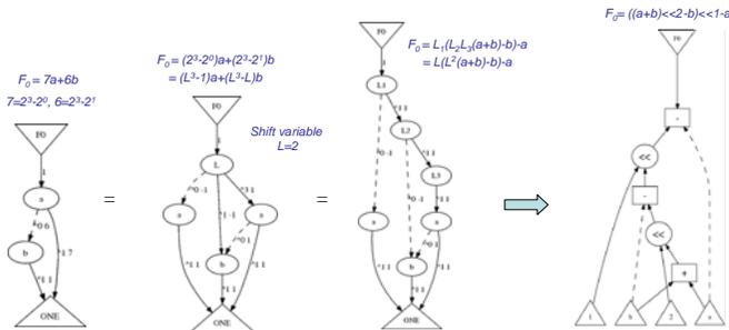
Fig. 4 Transforming TED with constant multiplications into DFG with shifters
