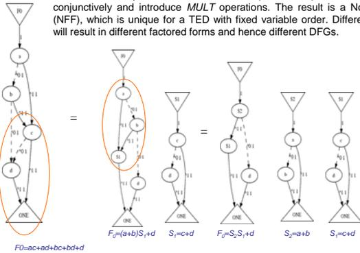
Fig. 2 TED decomposition leading to a unique Normal Factored Form:  $F_0 = (a+b)(c+d)+d$
