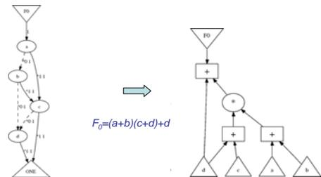
Fig. 3 Transforming TED into DFG based on Normal Factored Form obtained by TED decomposition
