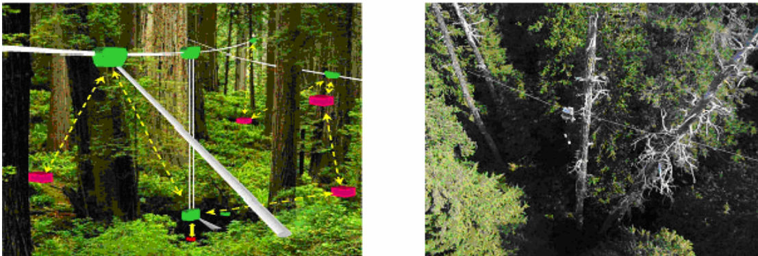
Figure 2: Examples of outdoor sensor network distributions depicting the difficult environments in which nodes need to work. On the left nodes in trees and on the forest floor monitor the habitat, on the right a node is hung from a wire fifty feet above ground.
