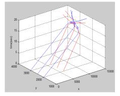
Figure 5: Simulation results for PNG, with a computer response of 0.01s. Blue (Red) lines are missile (target) trajectories. Once the missile enters its explosion range, it explodes, and this missile and its target stop moving.
