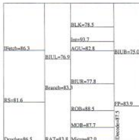
Figure 17: Pro-low: a floorplan with low maximum temperature for Pentium Pro
