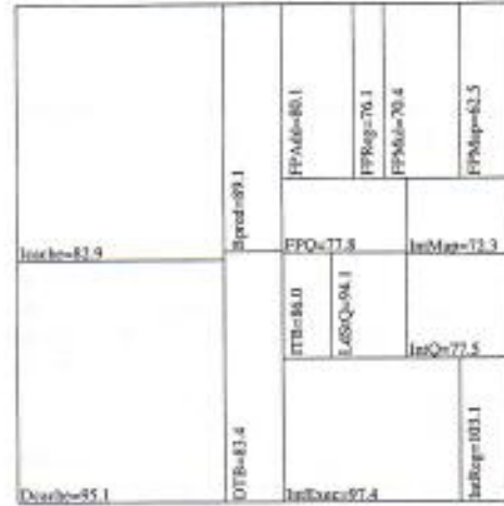
Figure 8: The block temperature ( ^{\circ}\text{C} ) for the rotated core Alpha floorplan
