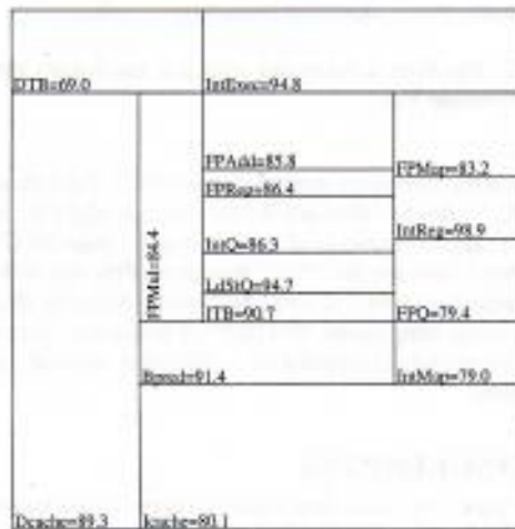
Figure 12: Wire-temp: a floorplan with both short wire length and low maximum temperature
