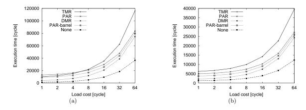
Figure 5: Execution times of AES with protection of all load instructions (a), and with protection of the load instructions in the last three rounds only (b)
