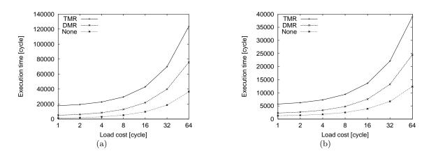
Figure 4: Execution times of AES with protection of all the instructions(a), and with protection of the load instructions in the last three rounds only (b)
