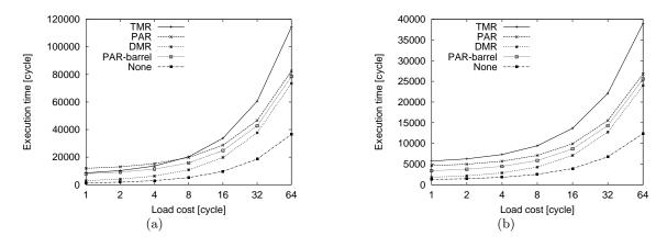
Figure 3: Execution times of AES with protection of all load instructions (a), and with protection of the load instructions in the last three rounds only (b) without cache flushing
