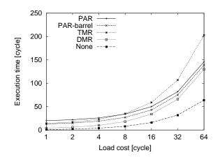
Figure 1: Time overhead required to protect a single load instruction as a function of the clock cycles needed to execute it
