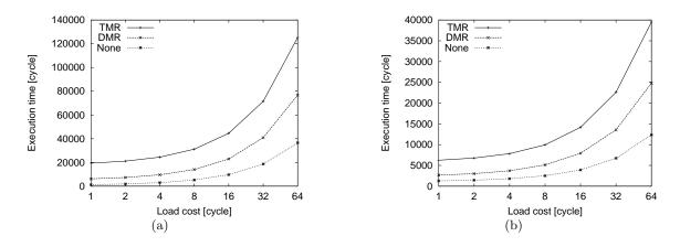
Figure 6: Execution times of AES with protection of all the instructions(a), and with protection of the load instructions in the last three rounds only (b) with cache flushing
