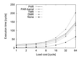
Figure 2: Time overhead required to protect a single load instruction as a function of the clock cycles needed to execute it including cache flushing
