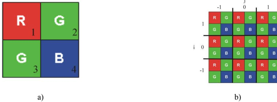
**Figure 2: a) Bayer Color Filter Array with  $k$  numbering; b) Pixel color array showing surrounding pixels with relative  $(i,j)$ .**
