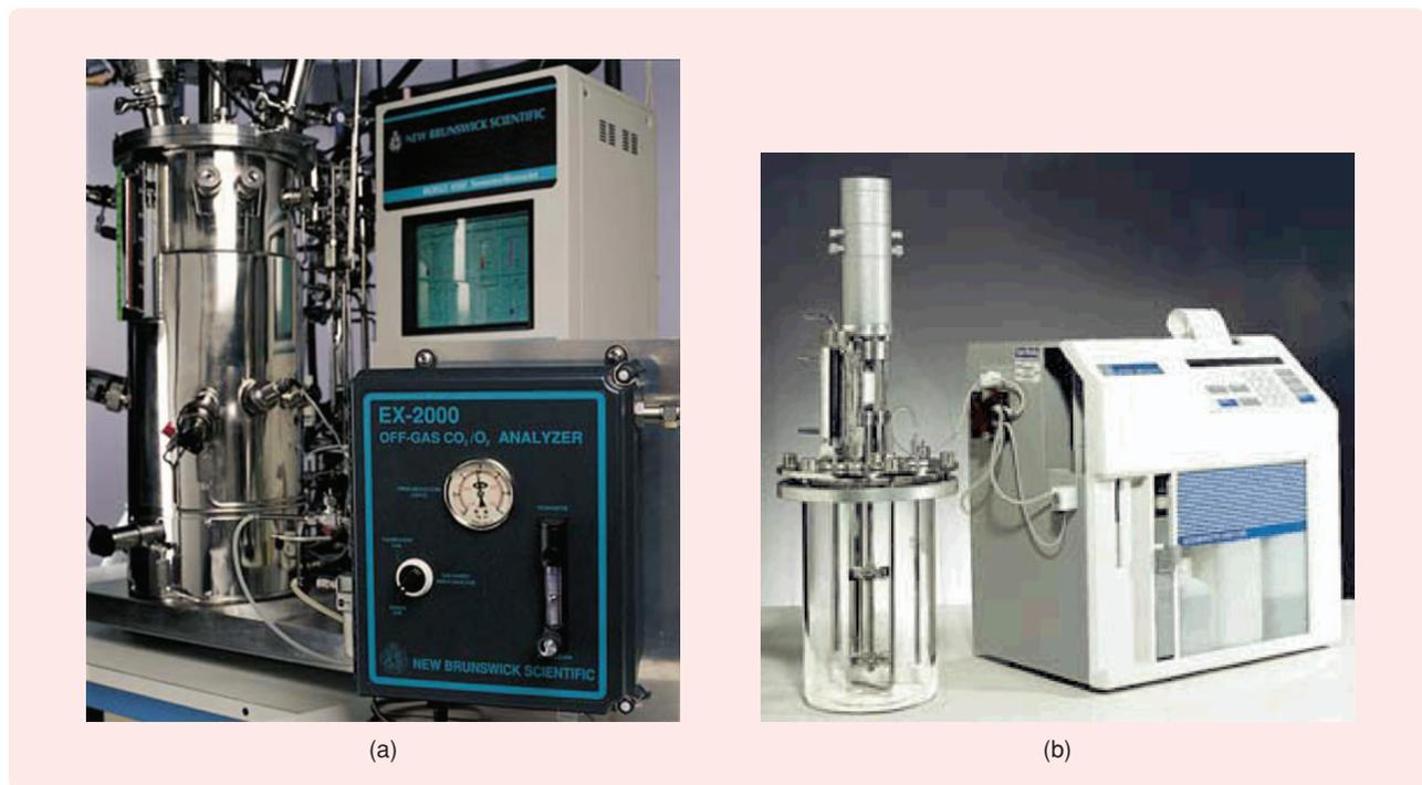
**FIGURE 3** Commercial technology for online measurement of bioreactor growth conditions. The exhaust gas analyzer in (a) provides continuous measurements of oxygen and carbon dioxide concentrations in the vapor space above the reaction liquid. (Courtesy of New Brunswick Scientific.) The biochemical analyzer in (b) provides online concentration measurements of two biochemical species such as glucose and ethanol in the reaction liquid. (Courtesy of YSI Incorporated.)
