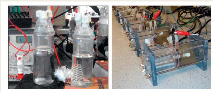
Bottle (left) and tubular (right) laboratory-scale microbial electrolysis cells.
