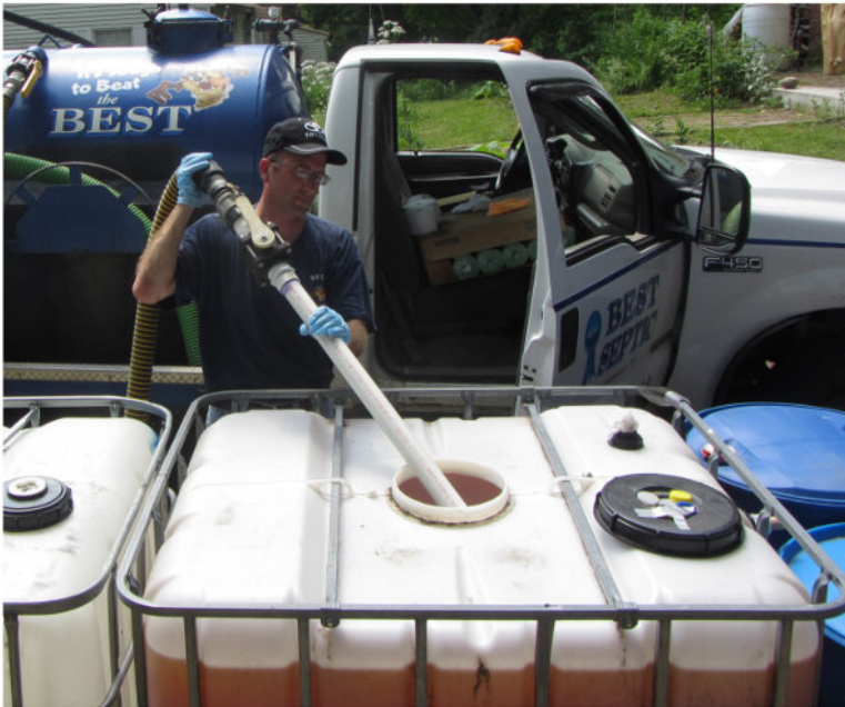
Figure 1. Pumping urine from the collection depot using a vacuum truck for transport to a participating farm.
