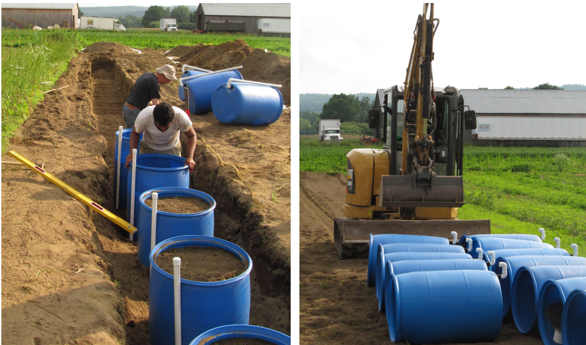
Figure 3. Installation of lysimeters to measure pharmaceutical and biological concentrations in soil leachate.
