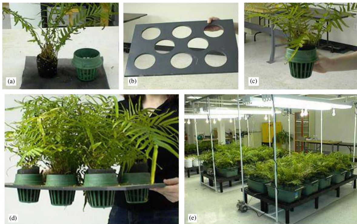
Fig. 1. Photographs of the principal components of the phytofiltration system, (a) plant in potting mix, foam wrap, and cup, (b) plant suspension tray showing location of eight plants per tray, (c) an entire wrapped fern plant, (d) tray of eight fern plants, and (e) bank of ferns in phytofiltration nursery system used to develop the root system of the ferns.
