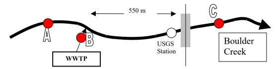
At 8:00 A.M. on December 29, 1994, conductivities of 170, 820, and 639  $\mu$ mho/cm were measured at A, B and C respectively. (Note: Conductivity provides an estimate of the total dissolved solids (TDS) in a solution by measuring its capability to carry an electrical current.) If the flow at the gaging station was 0.494 cms, estimate the flows for the treatment plant and the creek.
