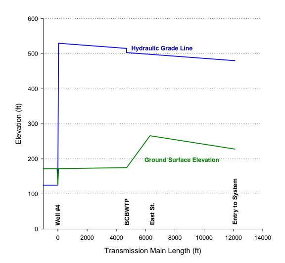
10. Calculate HGL and graph along with ground elevation and key system landmarks.
