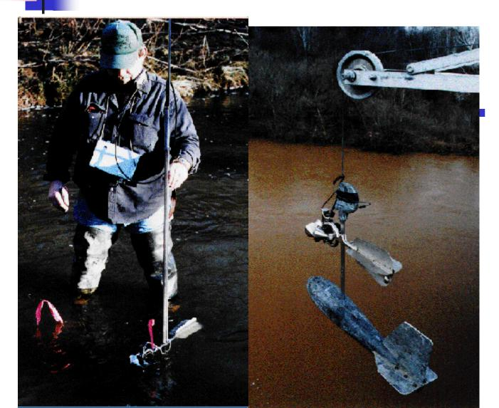
Current meter and weight suspended from a bridge crane
