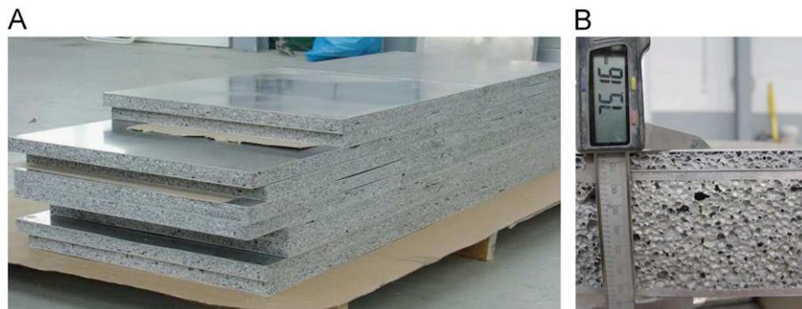
Fig. 2. Aluminum foam sandwich panels (a) on pallet, (b) in section [3]. (Photo credit: J Banhart).
