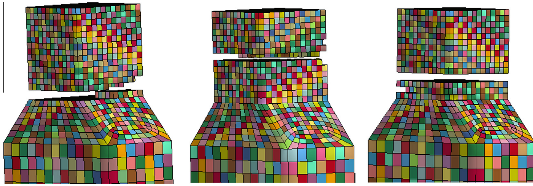
Fig. 11. Sample numerical realizations of tensile fracture. Note: colors represent model components with randomly assigned, unique material properties. Colors are cycled (due to limited number of available colors), thus two identically colored elements do not have the same material properties. (For interpretation of the references to color in this figure legend, the reader is referred to the web version of this article.)
