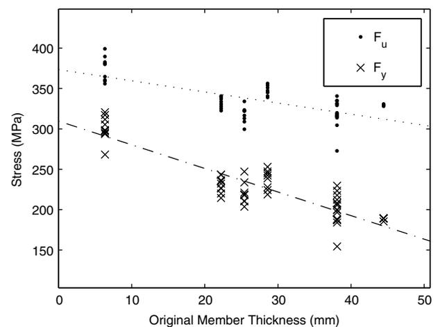
**Fig. 7.** Values of yield stress and tensile strength plotted against thickness of original member (1 MPa = 0.145 ksi and 1 mm = 0.04 in.)
