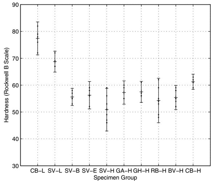
**Fig. 3.** Individual hardness values for each specimen group plotted with error bars
