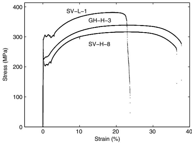
**Fig. 2.** Stress-strain curves of specimens SV-H-8, SV-L-1, and GH-H-3 (1 MPa = 0.145 ksi)
