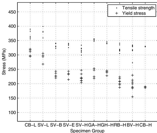
**Fig. 6.** Values of yield stress and tensile strength for each specimen arranged by group
