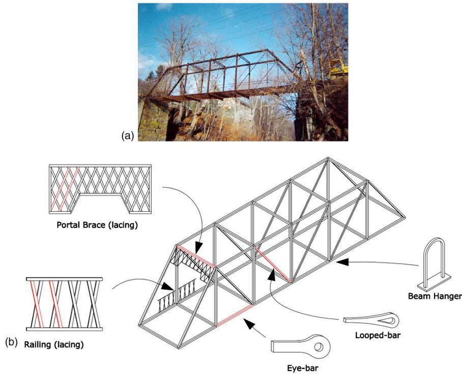
**Fig. 1.** Shattuckville, Massachusetts, bridge prior to dismantling and schematic member locations: (a) Shattuckville bridge prior to dismantling (photo by A. J. Lutenege); (b) relative locations on a schematic truss bridge of the different members sampled for testing (note that this drawing is a composite of the bridges studied that is designed to show the location of all members tested)
