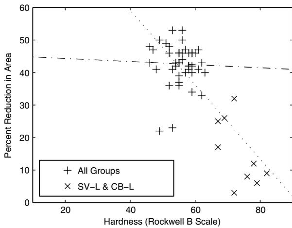
**Fig. 5.** Percent reduction in area plotted against hardness for each specimen with trend lines
