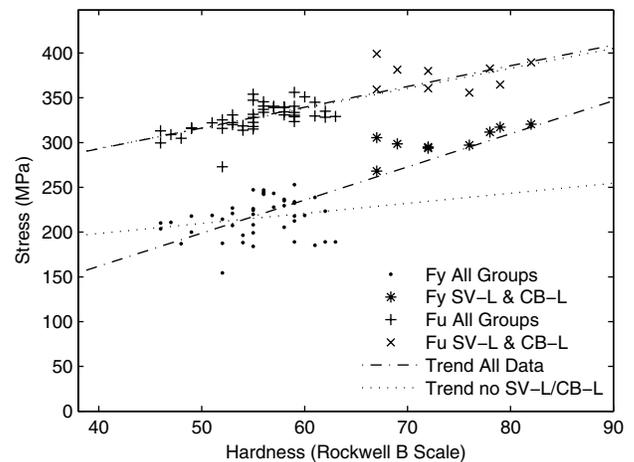
**Fig. 4.** Yield stress and tensile strength plotted against hardness with trend lines (1 MPa = 0.145 ksi)
