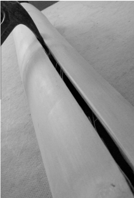
Fig. 2. Splitting Moso-bamboo culm.
