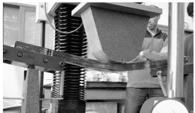
Fig. 10. Failed laminated bamboo lumber specimen in three-point bending.
