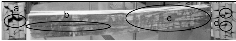
Fig. 6. LBL specimen that failed in horizontal shear due to a large longitudinal gap at the center of its cross-section; (a) Cross-section of specimen at its left end showing concentration of cracks at center; (b) Shear failure on left portion of specimen; (c) Right portion of specimen, which is not damaged; (d) Cross-section of specimen at its right end showing a critical concentration of transverse gaps in the layers.
