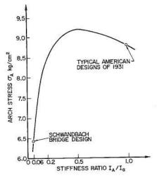
Allen Sit, an undergrad who is working with me, has developed a model in ADINA of a realistically dimensioned two hinged arch bridge. The figure shown below shows his ADINA results compared with Billington's equation. There is a discrepancy in magnitude that we are trying to work out, but the important part is that the peak in stress occurs at the same point,  $I_a/I_g=0.5$ , and the shape of the curves is the same.
