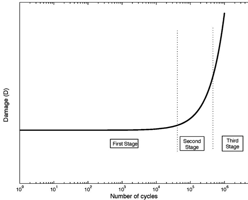
Fig. 2 Schematic damage accumulation curve.
