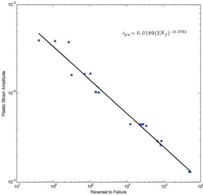
Fig. 4 S-N curve of the results published by Ingraham *et al.*<sup>11</sup> for plastic strain amplitude, using the Coffin-Manson model.
