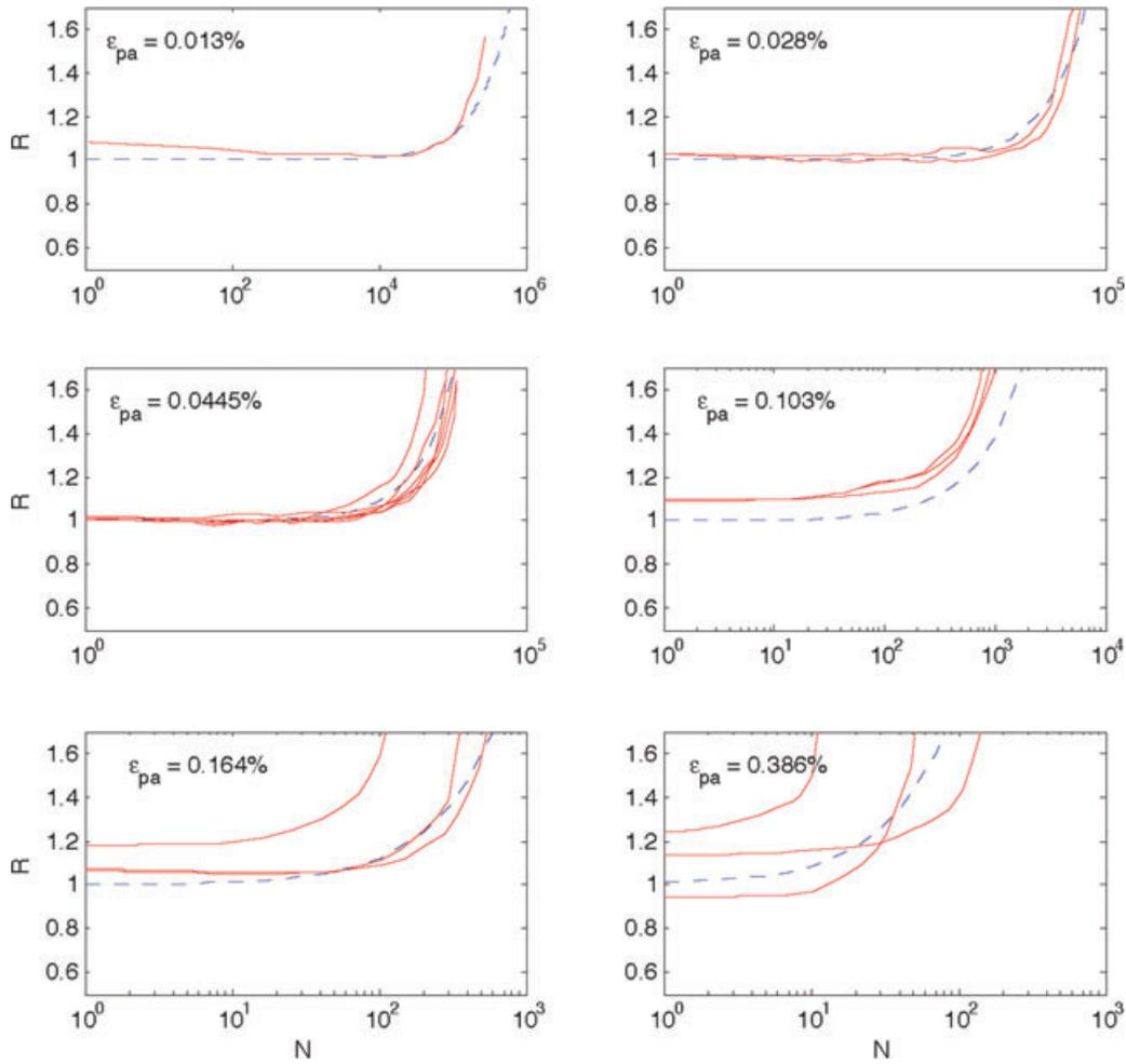
Fig. 8 Damage accumulation curves for different strain amplitudes obtained from the linear approach using the plastic strain amplitudes and the Weibull model.
