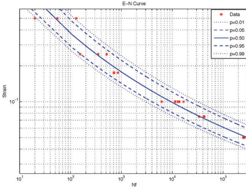
Fig. 10  $\varepsilon-N$  field curves of the results published by Ingraham *et al.*<sup>11</sup> using the total strain amplitudes.
