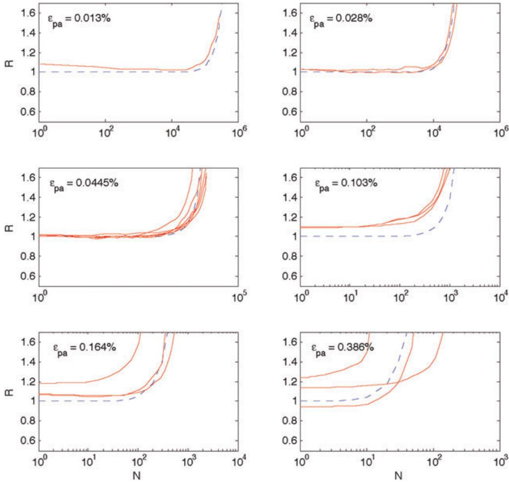
Fig. 6 Damage accumulation curves for different strain amplitudes obtained from the quadratic approach using the plastic strain amplitudes and the Coffin–Manson fatigue model.
