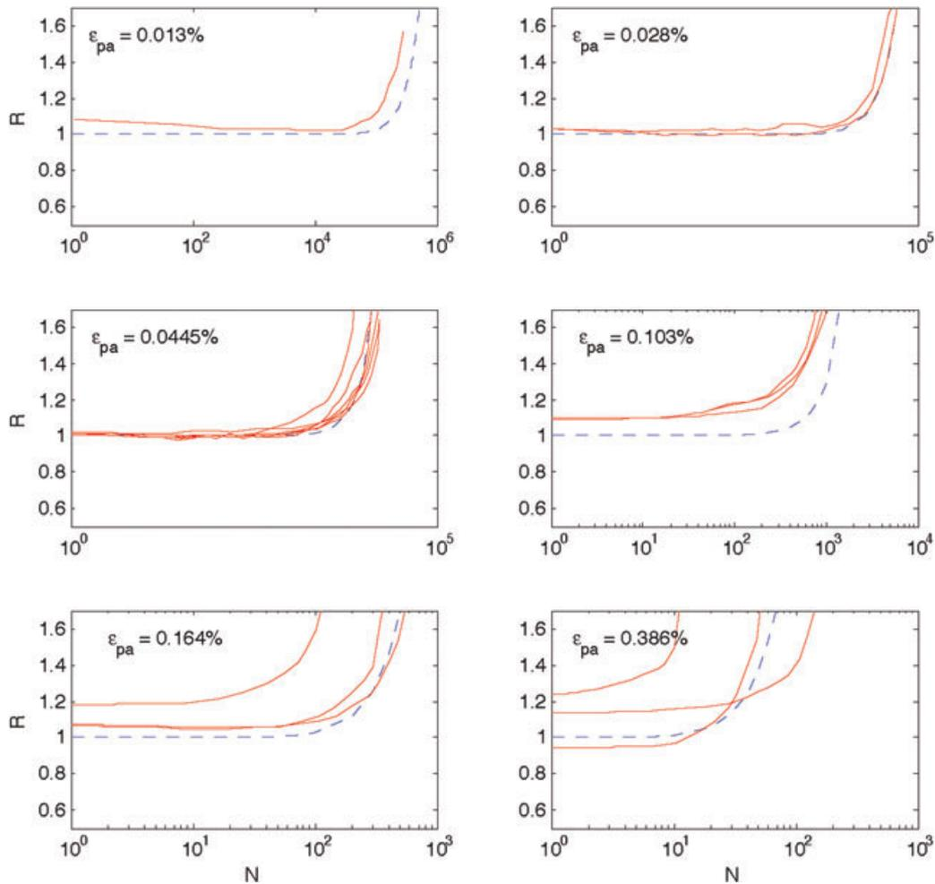
**Fig. 9** Damage accumulation curves for different strain amplitudes obtained from the quadratic approach using the plastic strain amplitudes and the Weibull model.
