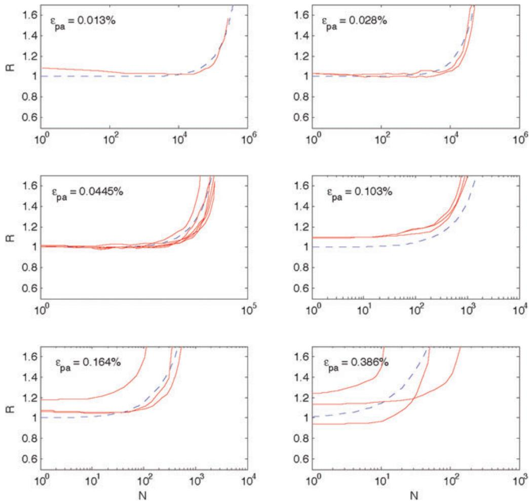
**Fig. 5** Damage accumulation curves for different strain amplitudes obtained from the linear approach using the plastic strain amplitudes and the Coffin–Manson fatigue model.
