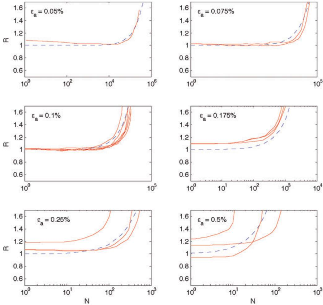
**Fig. 11** Damage accumulation curves for different strain amplitudes obtained from the linear approach using the total strain amplitudes and the Weibull model.
