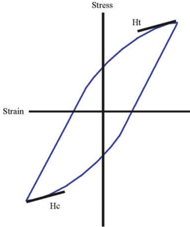
**Fig. 3** Schematic definitions of  $H_C$  and  $H_T$  according to Ingraham *et al.*
