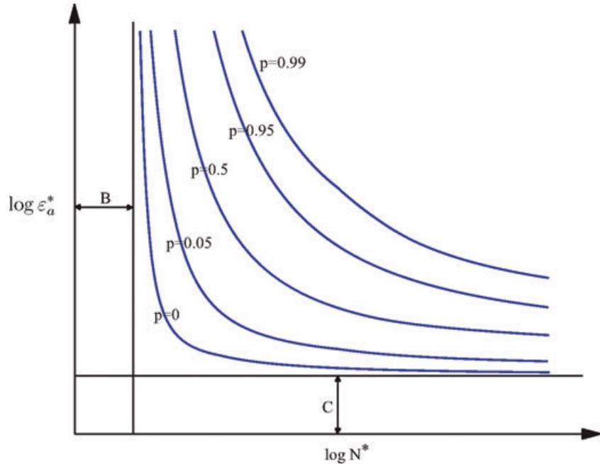
Fig. 1 Percentile curves representing the relationship between lifetime,  $N^*$  and strain range  $\epsilon_a^*$ , in the  $\epsilon-N$  field for the fatigue model.
