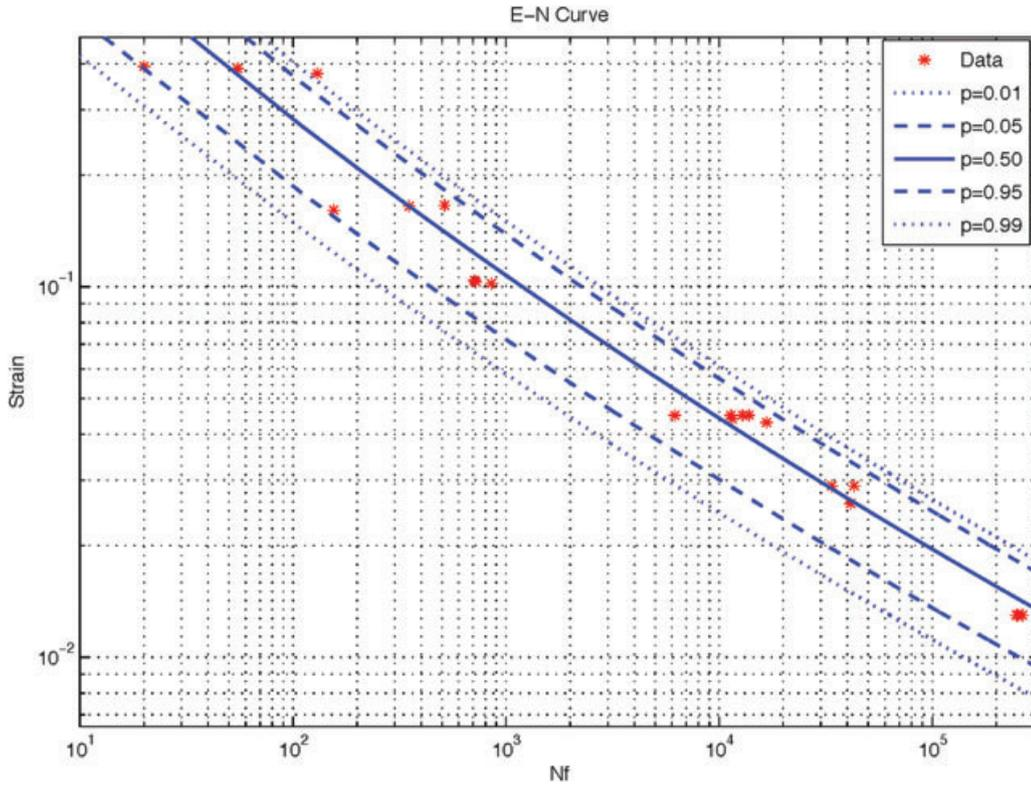
Fig. 7  $\varepsilon$ - $N$  field curves of the results published by Ingraham *et al.*<sup>11</sup> using the plastic strain amplitudes.
