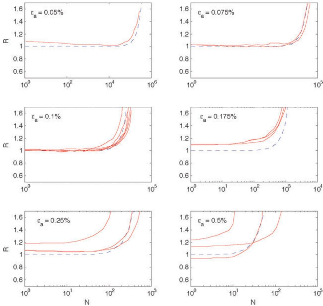
Fig. 12 Damage accumulation curves for different strain amplitudes obtained from the quadratic approach using the total strain amplitudes and the Weibull model.
