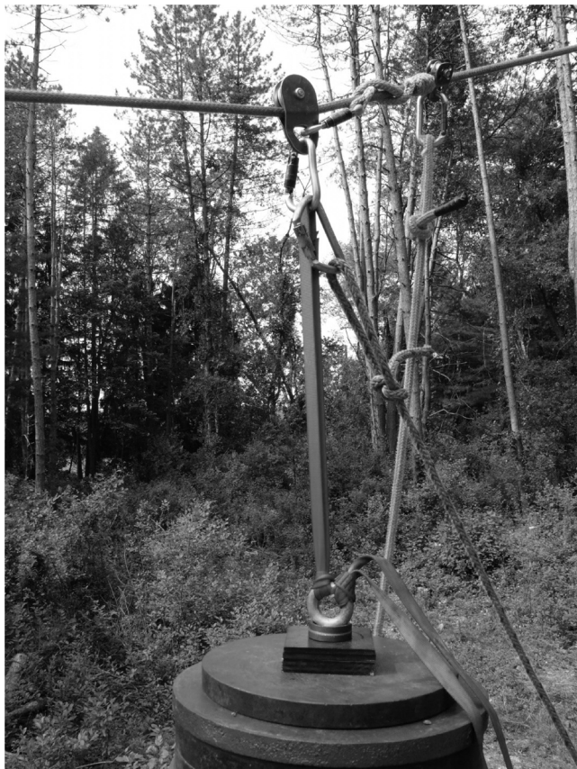
Fig. 1. Stack of weights hanging from a webbing sling attached to a pulley at mid-span of the speedline. The friction hitch and micro-pulley were used to position the stack at mid-span. The rope attached to the pulley holding the stack is the haul rope.
