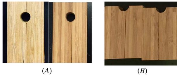
FE results. **Figure 4** illustrates the failure of the full- and half-hole dowel joints after being loaded in compression parallel to the grain up to their maximum stress.
