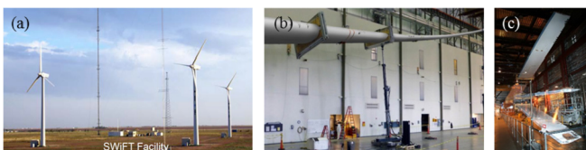
Fig. 9. (a) SWIFT Facility, Lubbock, TX [170]; (b) Flap fatigue test at Wind Technology Testing Center, Boston, MA-NREL from NREL Image Gallery #34756; (c) Inertial mass flap fatigue test at National Wind Technology Center, Boulder, CO, from NREL Image Gallery #16269 [182].
