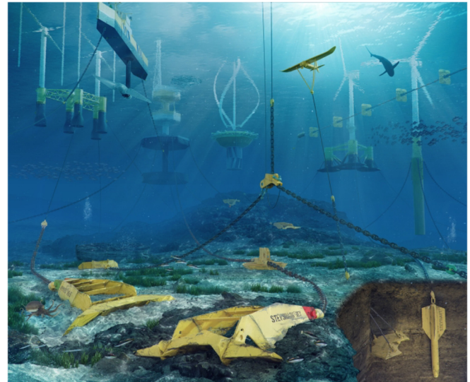
Fig. 4. Mooring and anchorage systems (Image courtesy S. Ozmutlu, Vryhof Anchors).
