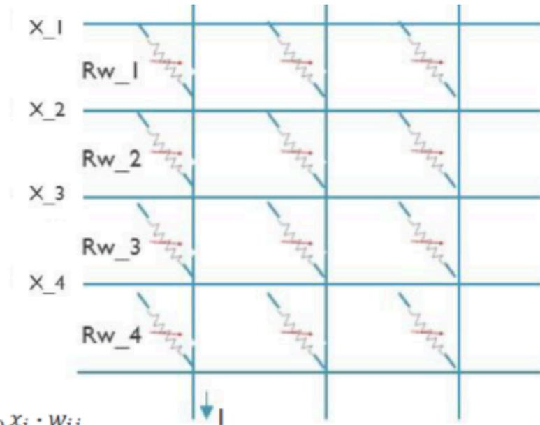
Figure 1: Analog Array.
