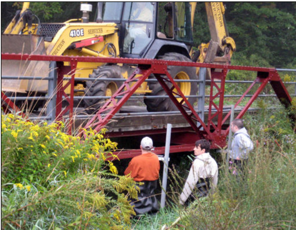
Figure 4. Adaptive use bridge team performing the load test.
