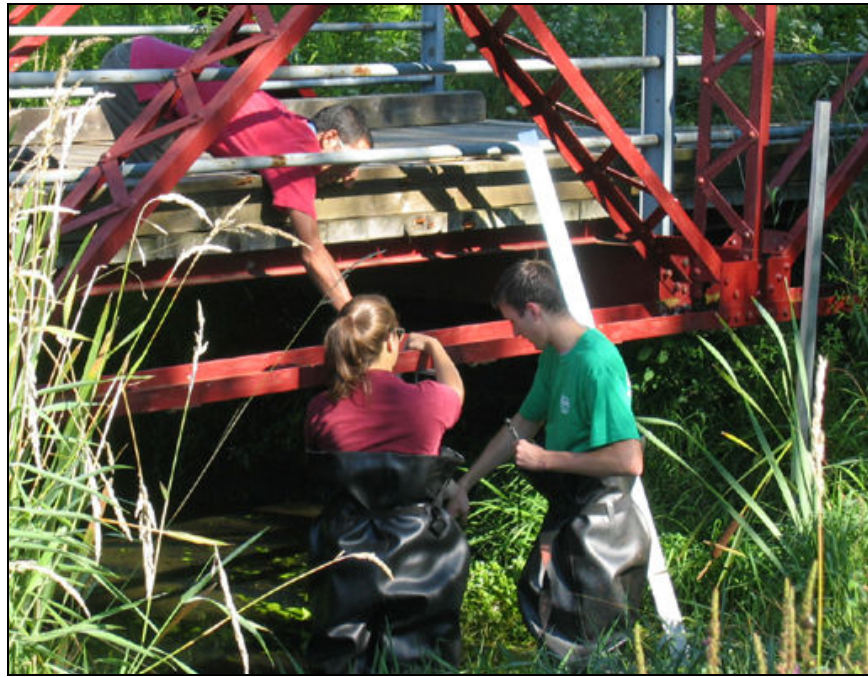
Figure 2. Members of the Adaptive Use Bridge Project team installing electronic dial gages on the Stadium Bridge.
