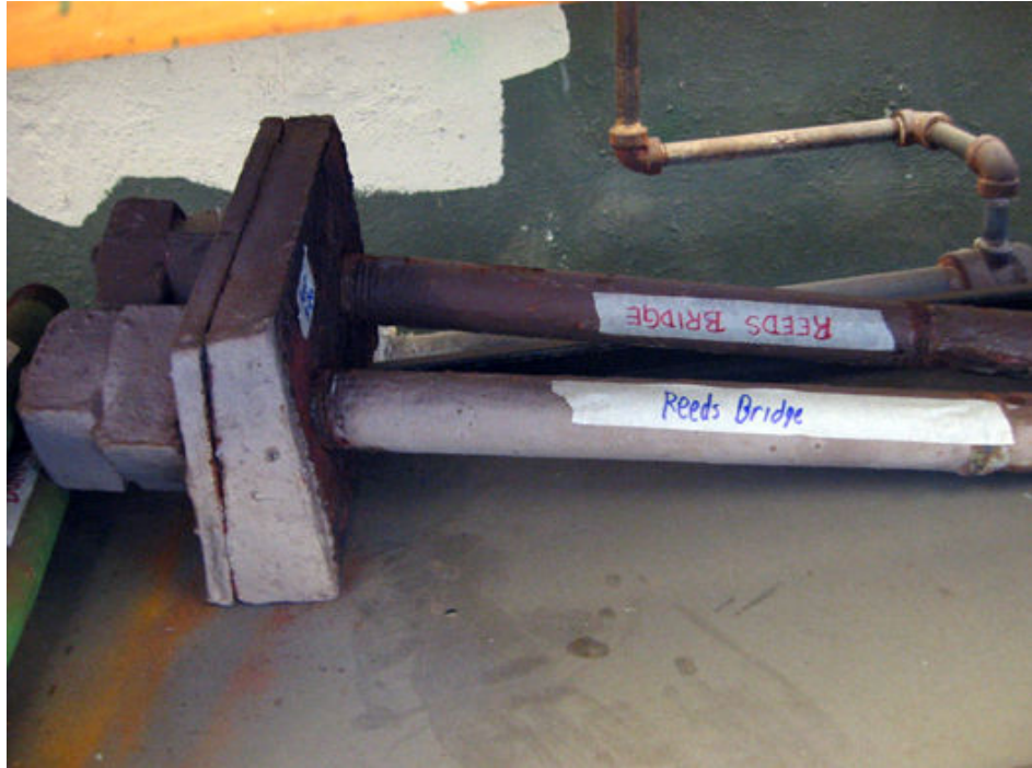
Figure 1. A Reeds Bridge Road Bridge beam hanger before being cut into several tension coupons.
