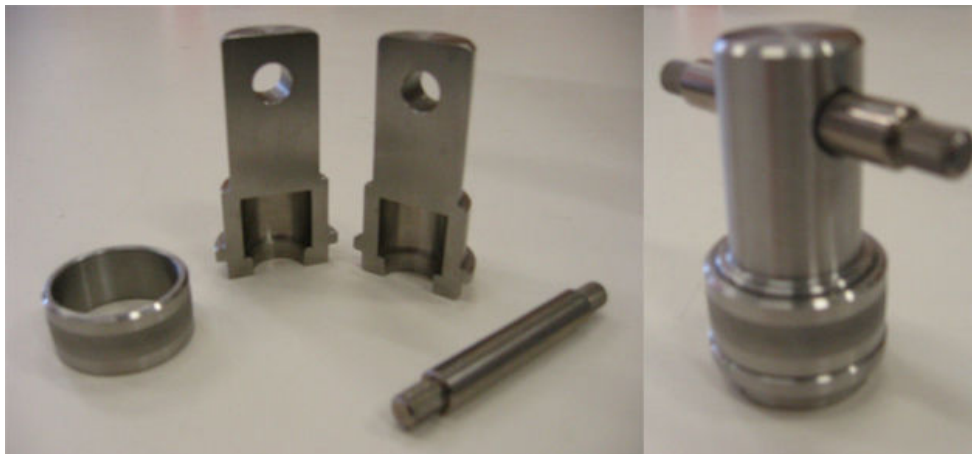
Figure 3. Custom made shoulder grips used to hold the tension coupons during testing.
