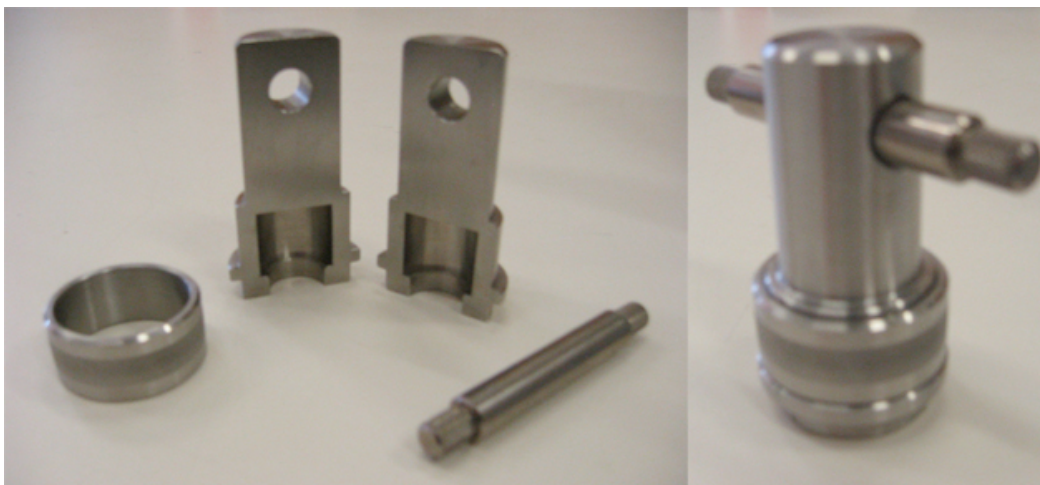
Figure 2. Custom made shoulder grips used to hold the tension coupons during testing.
